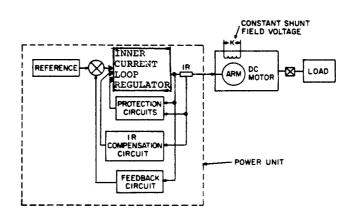
Figure 6-1. Block Diagram - Standard Drive with Armature Voltage Feedback
