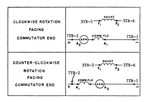
Figure 3-2. Shunt Motor
